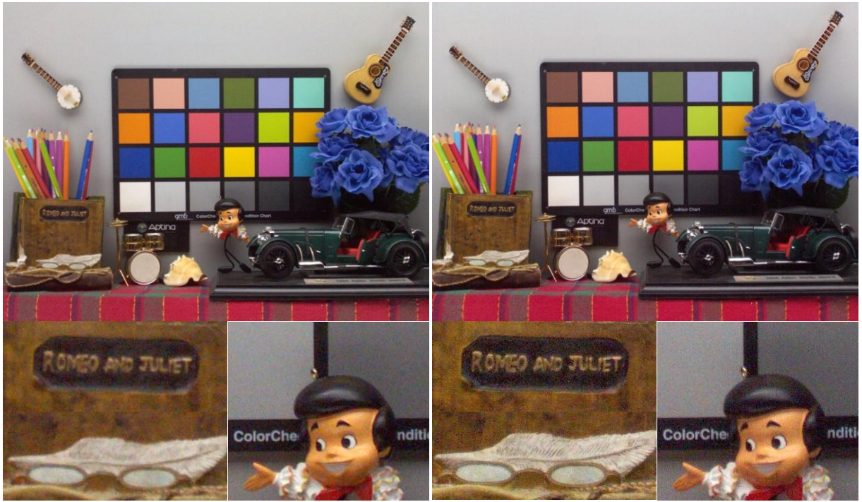
Figure 6. Image comparison between 5Mpix-1.4µm pixel (left) and 8Mpix-1.1µm (right) pixel at 100 lux scene illumination and 67ms integration time. Similar noise with sharper Image from 8Mpix-1.1µm sensor.
