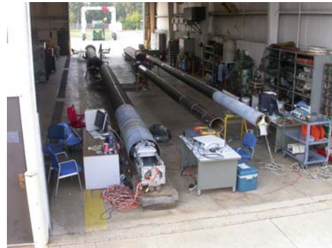
Figure 1 (left) north end of the high-bay area looking south. 30-inch SCC pipe and 24-inch mechanical damage pipe in foreground. Figure 2 (above) high-bay looking north. 12-inch corrosion and 24-inch mechanical damage pipe with gouges in foreground. Dent and gouge machine in far background outside the high-bay area.
