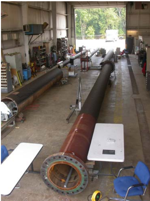
Figure 1 (left) north end of the high-bay area looking south. 30-inch SCC pipe and 24-inch mechanical damage pipe in foreground. Figure 2 (above) high-bay looking north. 12-inch corrosion and 24-inch mechanical damage pipe with gouges in foreground. Dent and gouge machine in far background outside the high-bay area.
