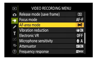
Scroll down to 'Attenuator', and press RIGHT.
